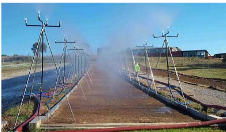
Figure 3. Rainfall simulation & erosion plot.
